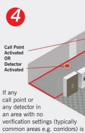
verification settings (typically common areas e.g. corridors) is activated, verification ends and a full fire alarm condition is immediately raised.
