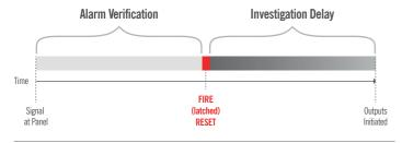
Verification and investigation comprise the two stages of complete false alarm management. Both are handled separately but configured in the same simple, powerful way using our AlarmCalm software.
