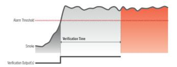
Signal not cleared, system in full fire condition at end of verification time.
