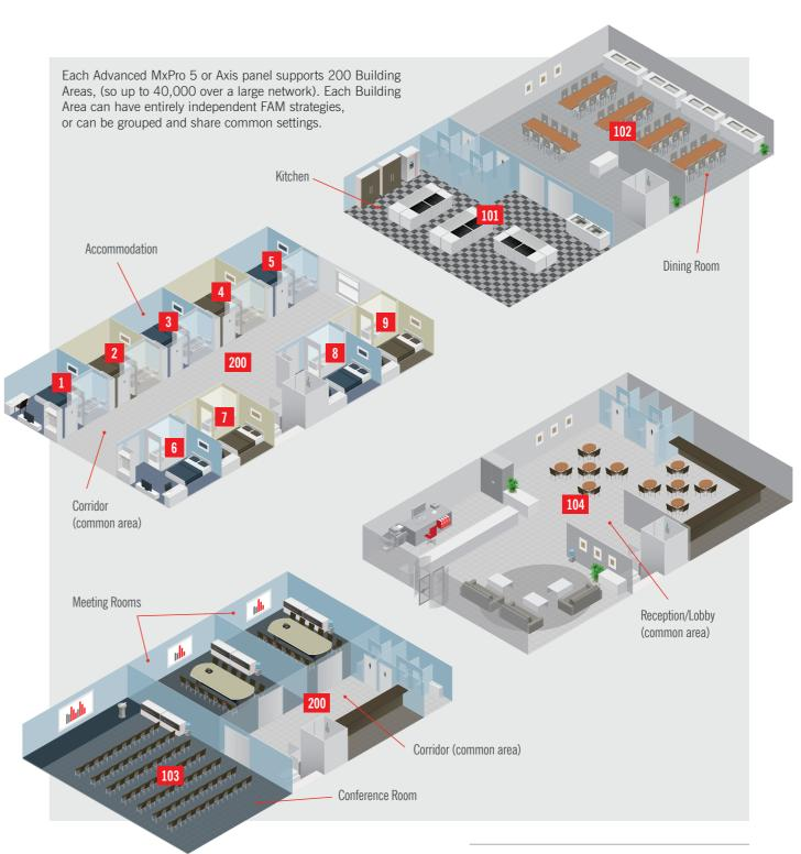
Each location within the building is allocated its own virtual building area number so that cause and effects can be programmed accordingly
