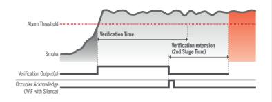
Signal remains above alarm threshold at end of 2nd Stage Time. System enters full alarm condition.
